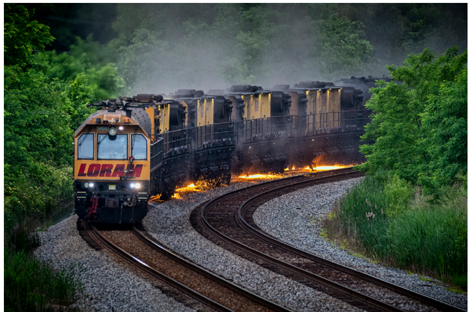
Right: LORAM Railgrinder RG414 grinds through a curve as it makes its way south at Nortonville, Kentucky on the CSX Henderson Subdivision on May 23rd, 2022. According to LORAM's Website: Rail grinding is the cornerstone of virtually every railroad maintenance program. It maximizes the life and value of rail assets through precision removal of fatigued metal, restoration of the rail head profile and removal of rail defects which are the optimization goals of an effective rail grinding program. Jim Pearson
